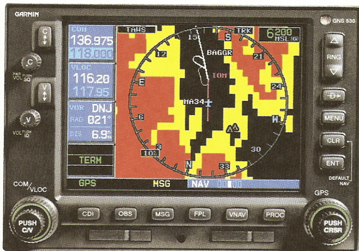
▲ Fig. 3-8 This is an air navigation GPS unit. It relates the plane’s location, as determined by GPS, to important information needed by the pilot.
